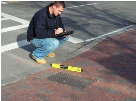
Recording ramp slope in field
